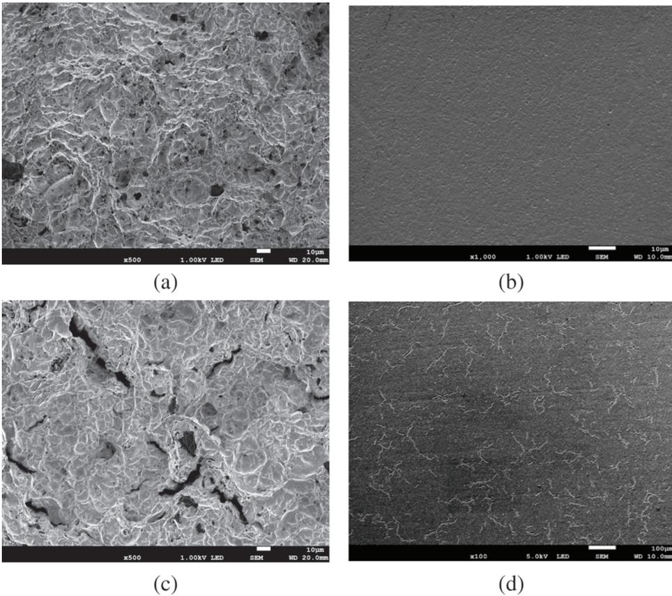
**Figure 3:** The cross-sections (a, c) and fracture faces (b, d) for the Zircaloy-2 alloy subjected to slow strain rate test: reference specimen (a, b) and after oxidation at 350 °C for 30 min, hydrogen charging and annealing (c, d).
