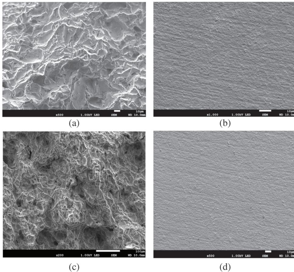
**Figure 4:** The cross-sections (a, c) and fracture faces (b, d) for the Zr 702 alloy subjected to slow strain rate test: reference specimen (a, b) and after oxidation at 350 °C for 30 min, hydrogen charging and annealing (c, d).
