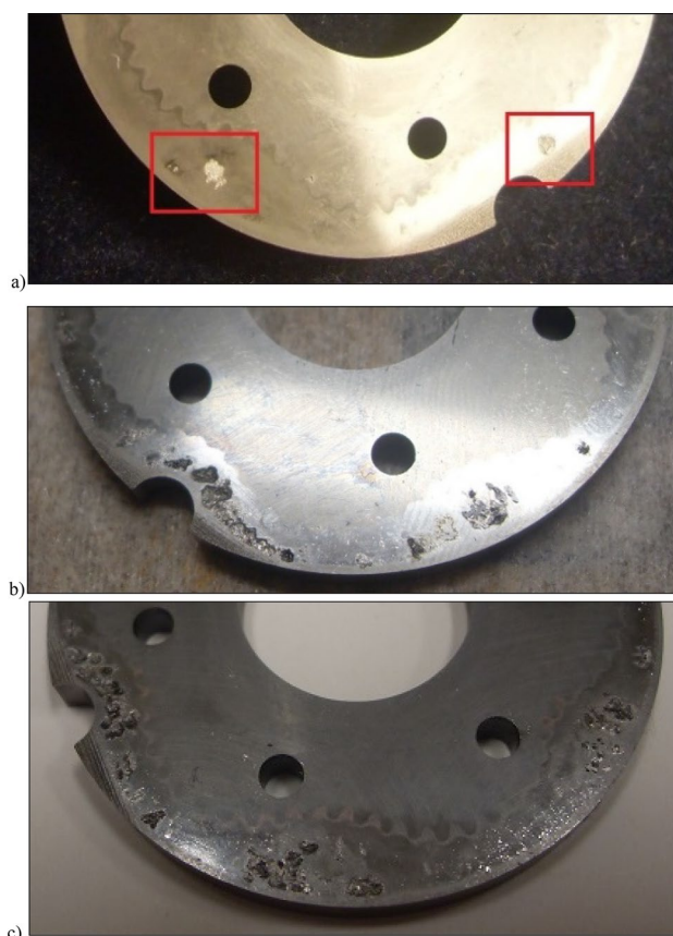
Figure 17. Fretting on the commutation plate: (a) after 11.5 min of operation; (b) after 1667 min of operation, (c) after completion of the test.
