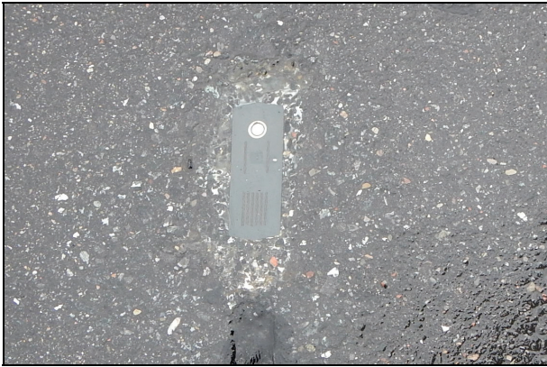
Fig. 4 Water film sensor on the test track in Horsens.
