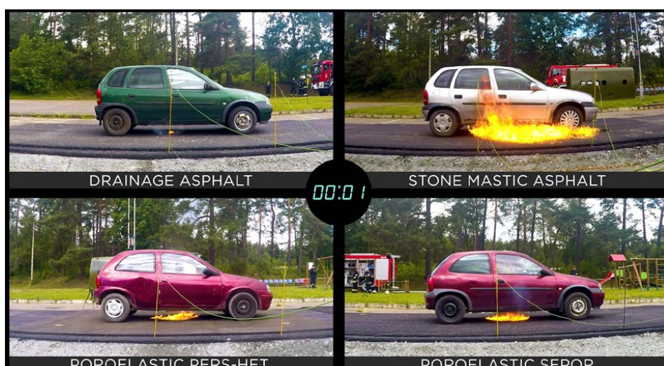
Figure 38. Development of fire 1 s after ignition.
