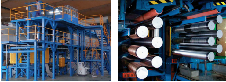
Figure 12. Single end cord production line and the pull roll section of this line [36]
