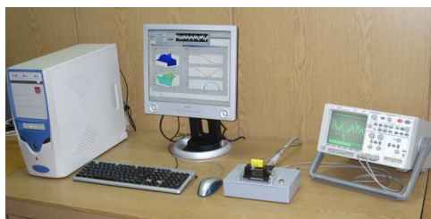
Fig. 5. View of the setup with an experimental impedance analyzer.
