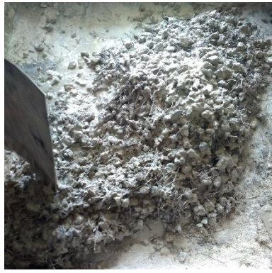
Fig. 1 Mixing of the HFRGC
