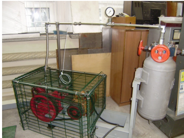
Fig. 3. General view of the Espholin H3S piston compressor test stand
