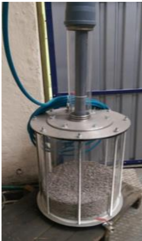
Fig. 3. View of lower tank
