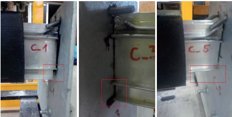
Fig. 10. Form of bracket failure under cyclic tests – visible displace of bottom aluminium profile
