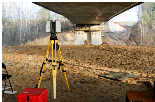
Fig. 10. Laser scanner Leica P30 station.
