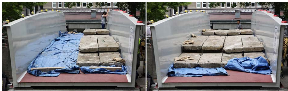
Figure 5. Footbridge loaded with ballast during static tests
