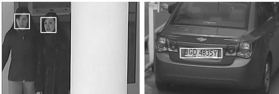
Figure 9: Results of face detector (left) and plate detector (right)
