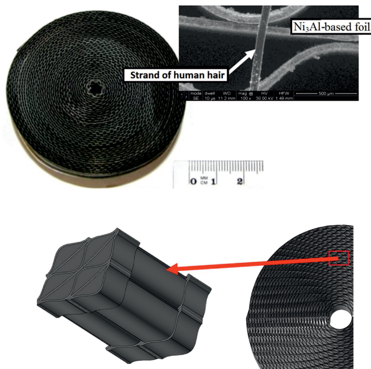
Figure 1: The alloy foil package based on the \text{Ni}_3\text{Al} intermetallic phase rolled into a honeycomb with zoomed foil and geometry of the eight single microchannels beginning at inlet into the package and terminating at the outlet from the package.
