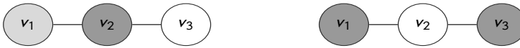
FIGURE 3 Two primary controllers placements and their resilience to a 1-node attack (linear metric)
