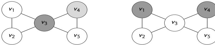
FIGURE 4 Two primary controllers placements and their resilience to a 1-node attack (quadratic metric)
