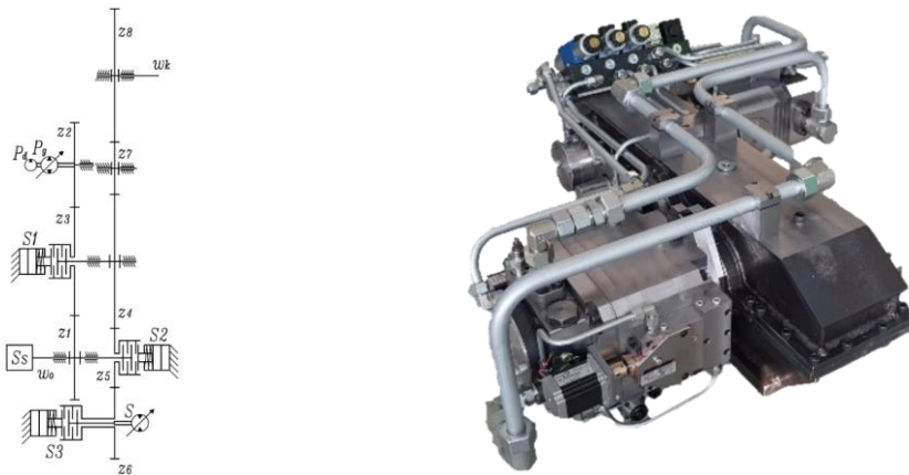
Fig. 1. Kinematic scheme and photo of hydromechanical gearbox
