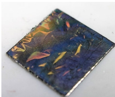
Figure 7. The nanodiamonds structure deposition on the tantalum substrate.
