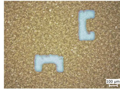
Fig. 5. Printed gold paste ground plane with C-holes with a structure width of 100 \mu\text{m} using a very fine resolution screen.
