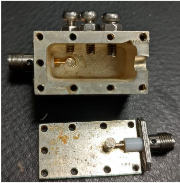
FIGURE 13. Photograph of the manufactured prototype of triplet filter with a TZ below the passband.
