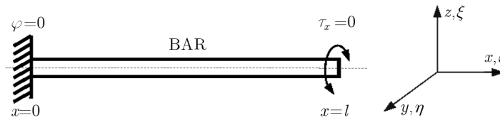
Fig. 4. Bar element (longitudinal vibrations) with exemplary boundary conditions, corresponding equation and bond graph representation, M_x – multiport representing the distributed parameter element, \zeta, \eta, \xi – displacements in x, y and z directions, respectively, f_x – force, s – Laplace operator, S_f – source, E – Young modulus, \rho – mass density, A – cross-sectional area, \delta – Dirac delta
