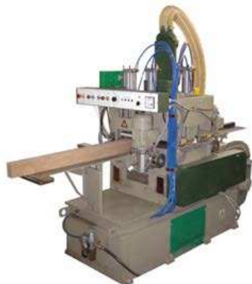
Fig. 4 Sash gang saw PRW 15 M.
