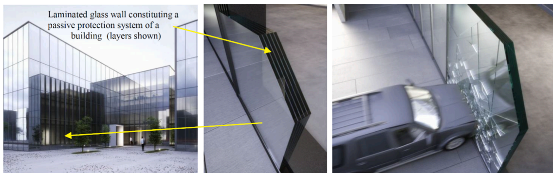
Fig. 14. An example of using a laminated glass wall that is a passive building protection system – visualization. (author’s own project).
