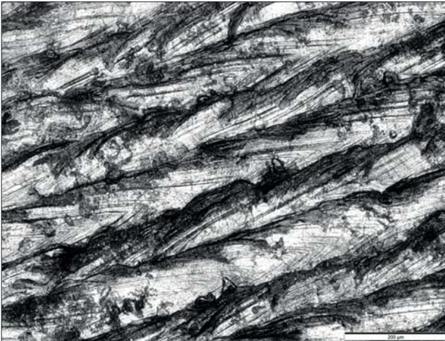
Fig. 3. Part of the surface of a workpiece made of MS1 material by DMLS: (a) a microscopic image of a real surface using OLYMPUS BX51; (b) digital model of the surface obtained with computer tomography
