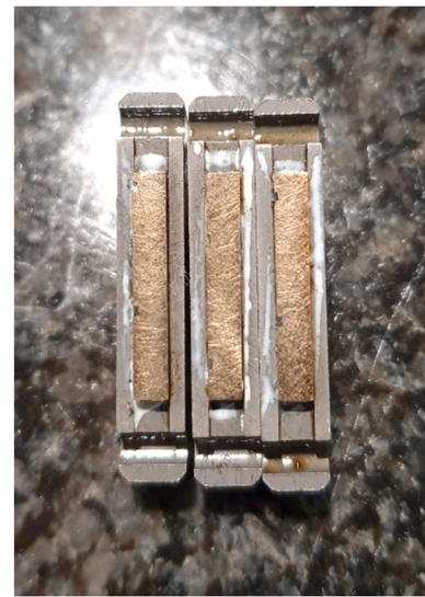
Fig. 3. cBN abrasive stones with metallic bond.
