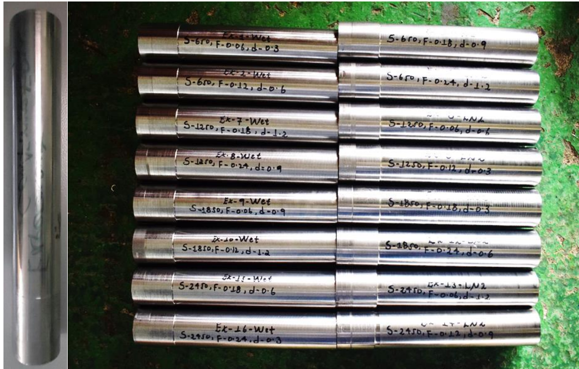
Figure 3. Samples of D2-steel after machining
