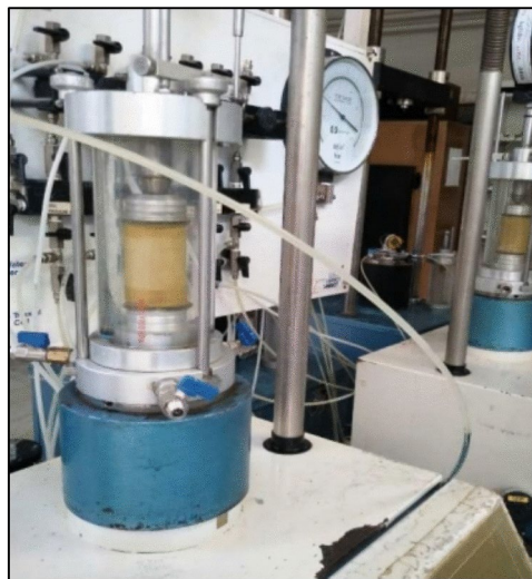
Fig. 4. Sample tested in the triaxial (UU) device.
