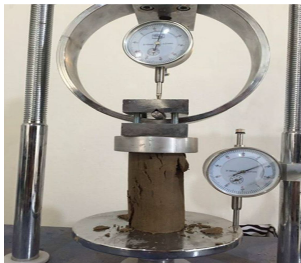
Figure 4. Specimen image after the UCS test.
