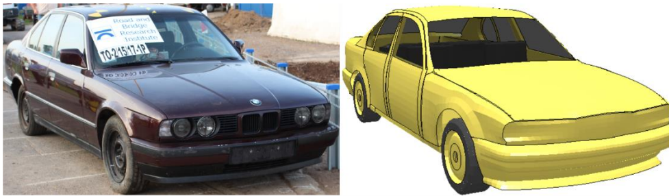
Fig. 4 Comparison between BMW car and its numerical model
