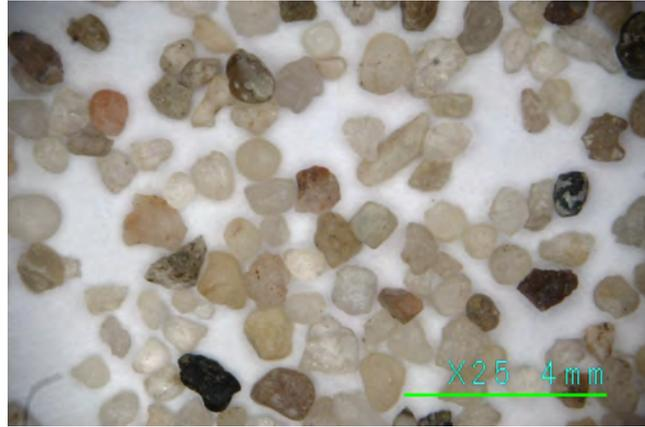
Figure A.5: Exemplary photograph of dry cohesionless sand used in the experiments.
