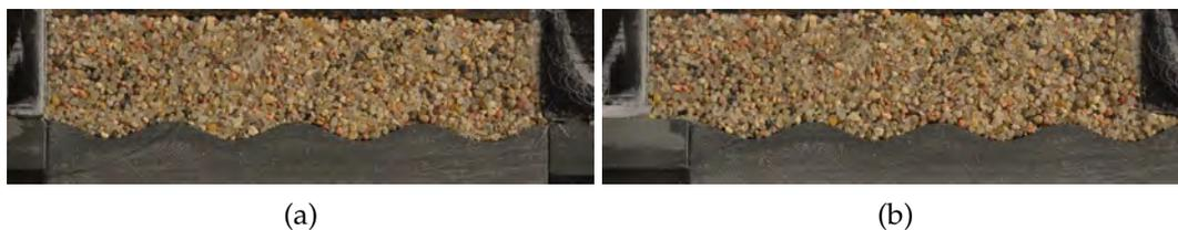
Figure A.6: Front view of the sand sample: a) prepared for the interface shear test and b) at the final state of the test for exemplary surface with corrugation coefficient  $d/l=0.147$ .
