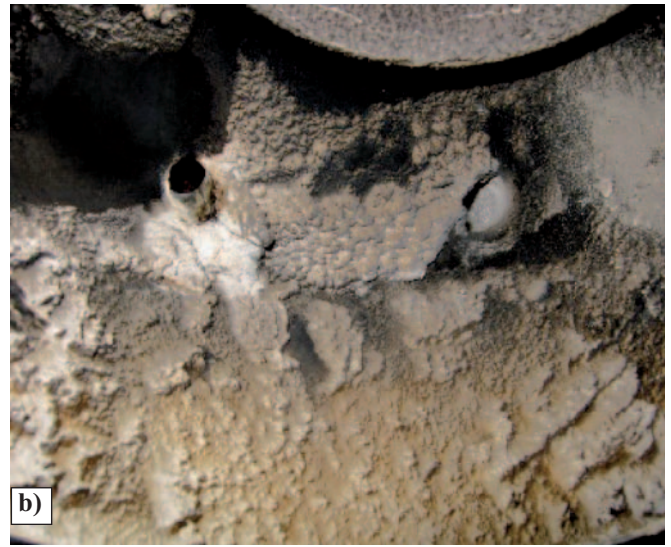
Fig. 3. View of cylinder space of the engine working on a biofuel produced on the basis of crude (not processed) palm oil.
