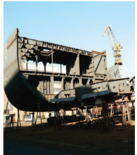
Fig. 2. Prefabricated ship's hull units and blocks in positions in which they are measured
