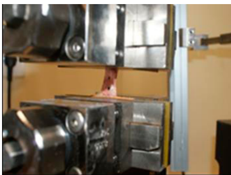
Figure 1. Mechanical bone examination using a Zwick Z020 strength testing machine with a video extensometer
