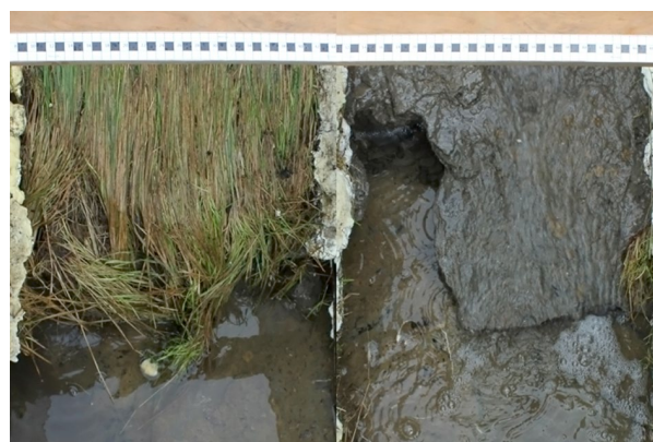
Fig. 17. Dike toe. Clay liner underneath the dike, slip line between the ash/silt dike cover and the clay base. Test section 9 of flume 1 (right) and flume 2 (left) after the 5 th TD (veg.)
