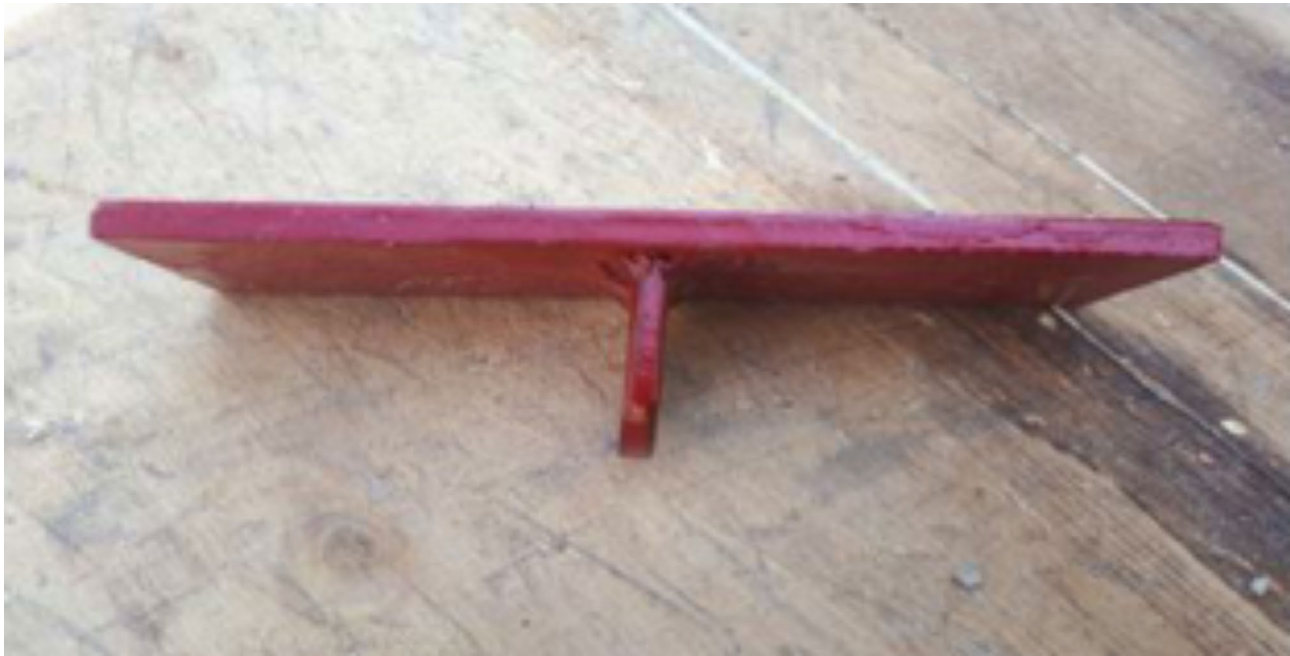
Fig. 2. Steel plate anchors used in the present research.
