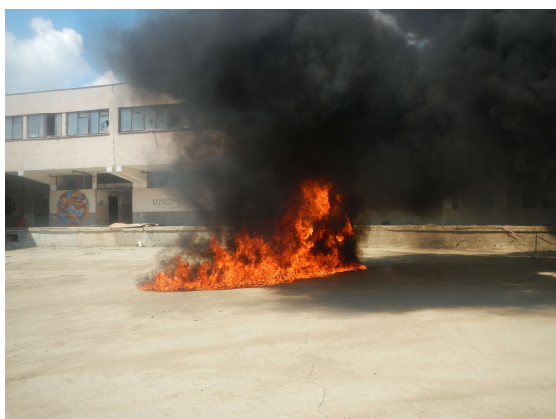
Fig. 9. Fuel fire on dens surface (after 10 s).
