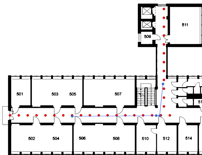
Fig. 19. Map of route points estimated by deep neural network models for the 'WiFi115' input vector (blue colour)
