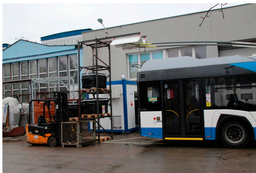
Figure 2. Technical tests of a prototype of a 150 kW fast charging station for trolleybuses in Gdynia (photo taken by M. Bartłomiejczyk).
