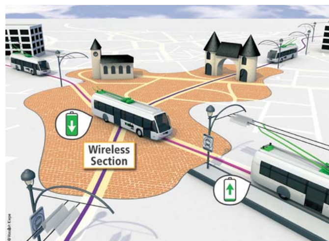
Rys. 1. Idea systemu In Motion Charging (IMC) [© Vossloh Kiepe]
