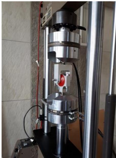
Figure 3 Specimen during fatigue test (80 ShA)
