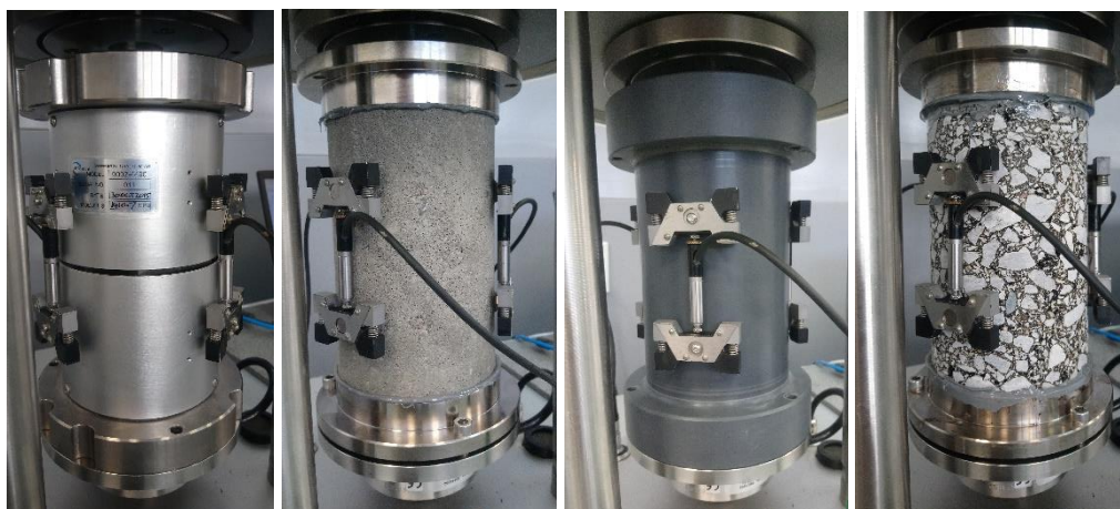
Fig. 3. Specimens used for verification of the test procedure (from left): steel dummy specimen, cement concrete, PCV and asphalt concrete.
