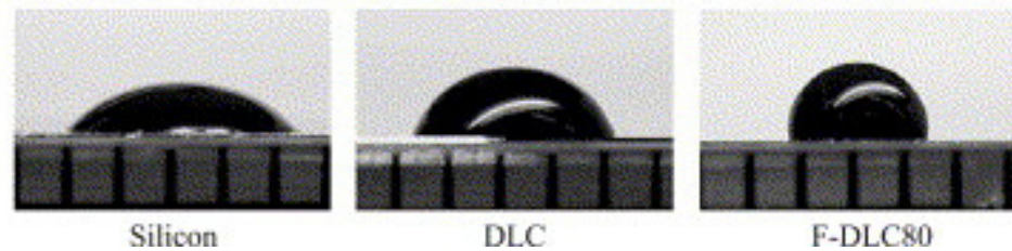
Figure 3. Contact angle measurements of 10 \mu\text{L} human whole-blood droplets on the sample surface. F-DLC80 showed the highest hydrophobicity (reprinted from [61], permission from Elsevier, license number 5510710188982).
