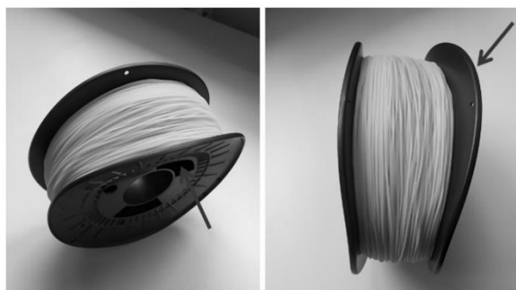
Figure S1. Damaged spool of TPU filament due to excessively high extrudate stresses generated during forming and winding process.
