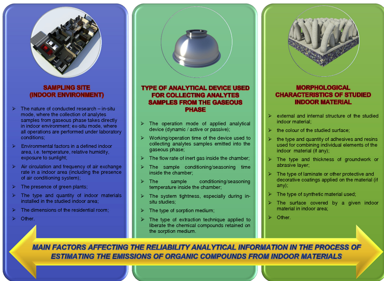
Fig. 8. Factors significantly affecting the reliability of data obtained when estimating emissions of chemical compounds released from indoor materials.
