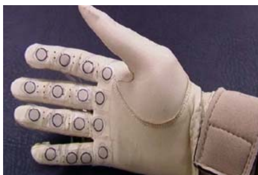
Fig. 2. Finger force measurement system (volar side) [3]
