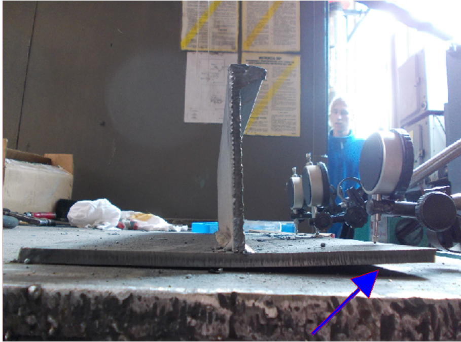
Fig.4. Measurement of angular deformation
