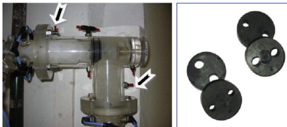
Figure 8. Examples of orifices used when measuring the degree of filling by means of a pressure drop in an orifice [4,10].
