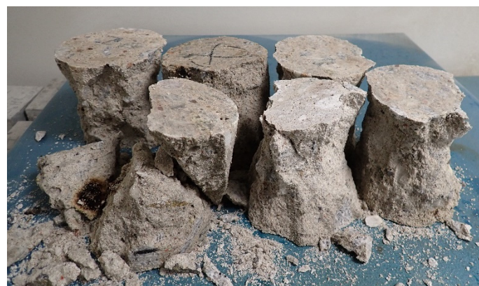
Figure 6. Parts of some concrete specimens after uniaxial compressive tests—views of the form of failure with visible organic inclusions and predominance of fine aggregates.
