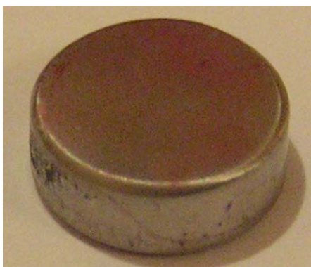
Fig. 6. Appearance of alloy surface after an exposure in Staphylococcus epidermidis solution
