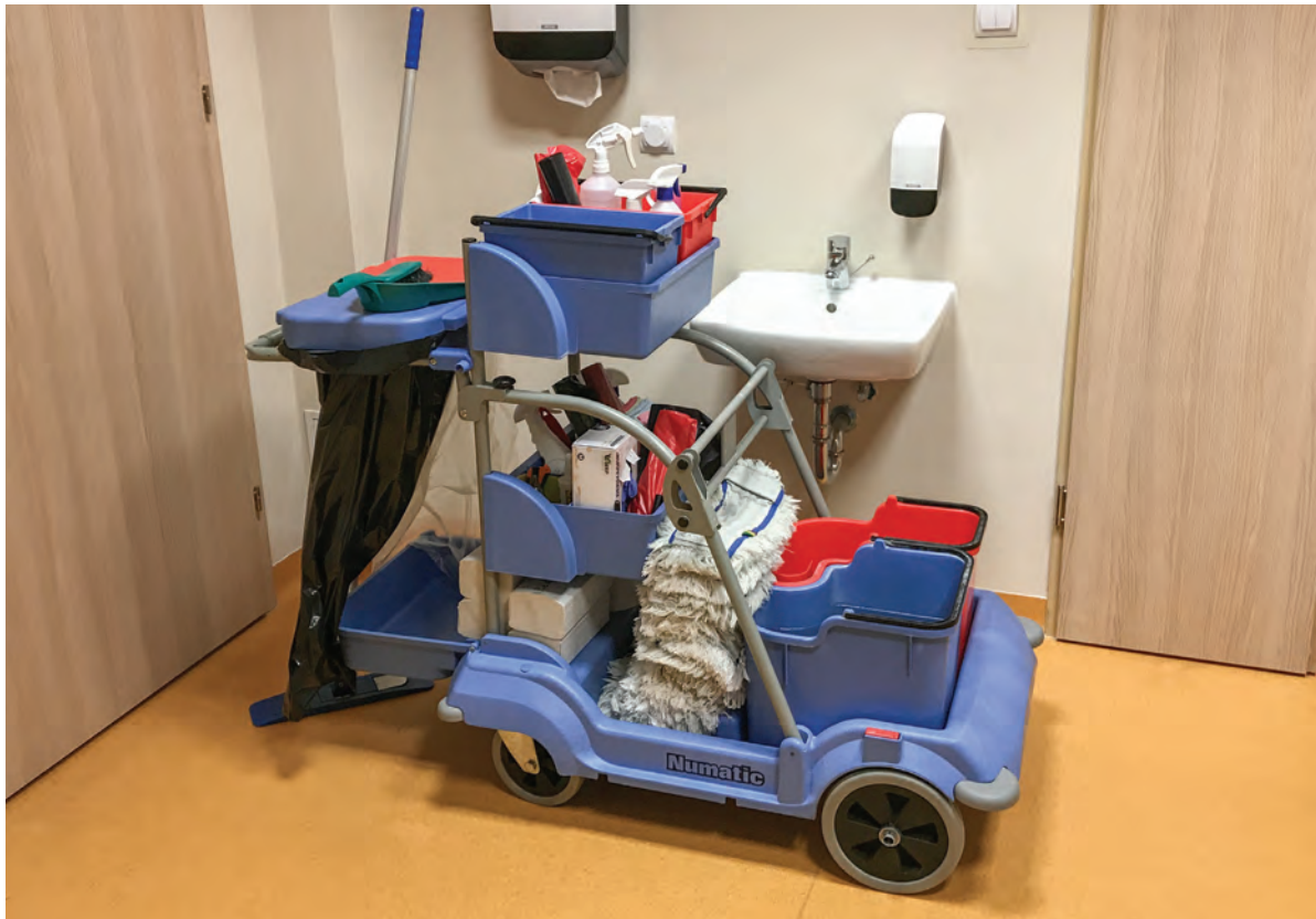
Photograph 6.5 A sanitisation trolley (the sanitisation process involves moving sanitisation equipment into the rooms in order to provide efficient performance of the sanitisation procedures); photographed by the Author 2018
