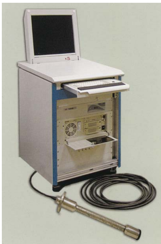
Fig.1 The parameter's controller of acoustic disturbance sources generated by a moving ship
